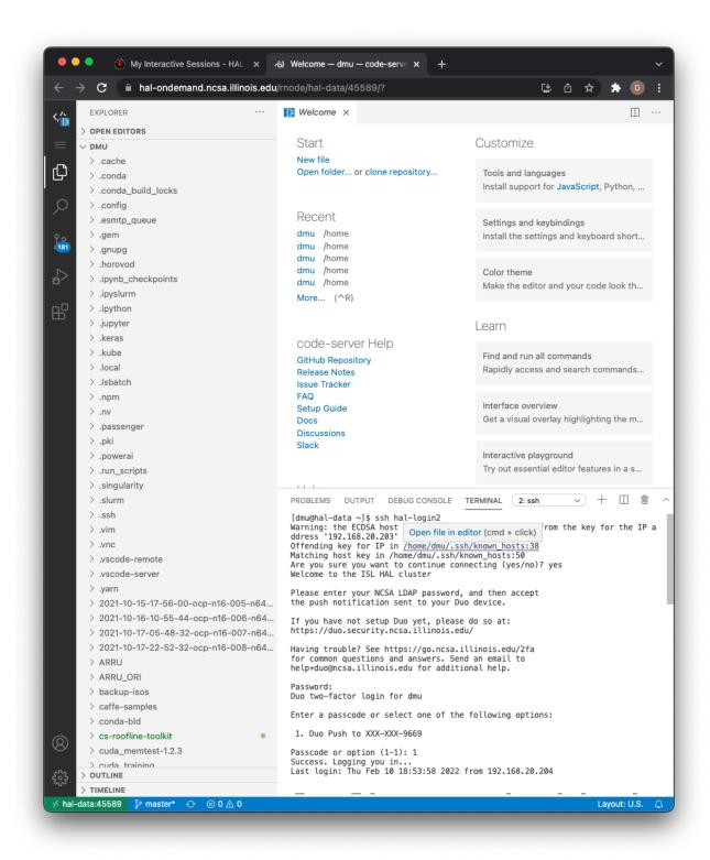
Request GPU Resources with **swrun -p gpux1** and load the python module with **module load opence**
