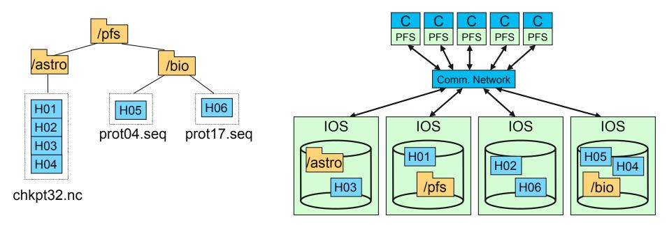
An example parallel file system, with large astrophysics checkpoints distributed across multiple I/O servers (IOS) while small bioinformatics files are each stored on a single IOS.
