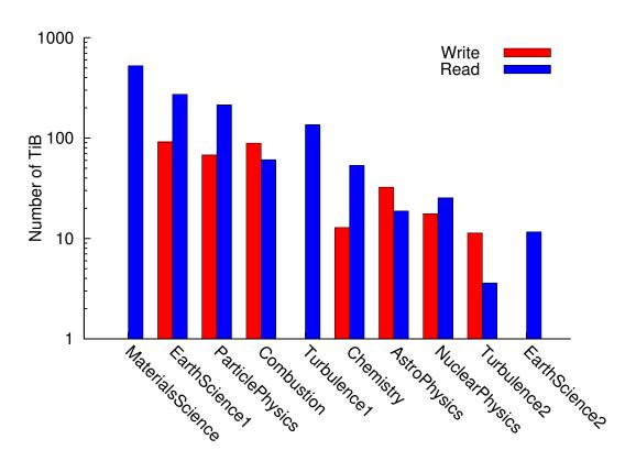
Top 10 data producer/consumers instrumented with Darshan over the month of July, 2011 on Intrepid BG/P system at Argonne. Surprisingly, three of the top producer/consumers almost exclusively read existing data.
